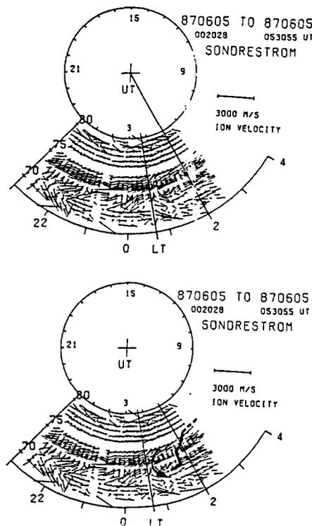
Fig. 3. F-region ion convection measured by the Sondrestrom radar in a clockdial format with UT measured around the inner circle and geographic LT measured around the outer circle. In the bottom panel we add schematic markings on the data to aid the viewer in observing the features described in the text.
