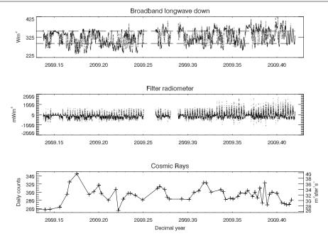
**Figure 2.** Time series of typical data, from 16 February–6 June 2009 showing (upper panel) broadband longwave down (5 min averages) with the upper  $(354 \text{ Wm}^{-2})$  and lower  $(295 \text{ Wm}^{-2})$  quartiles as horizontal dashed lines. The middle panel shows the filter radiometer signal (5 min averages), and the lower panel presents the raw muon flux, not temperature or pressure corrected, as both daily counts (left hand axis) and mean flux (right hand axis).
