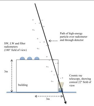
**Figure 1.** Schematic arrangement of the experiment, (not to scale) showing the radiometers mounted on a building and the adjacent cosmic ray telescope. The telescope can detect particles in a cone  $11^{\circ}$  from the vertical, with the geometry implying that approximately half the particles detected have passed over the radiometer at a height of >15 m.
