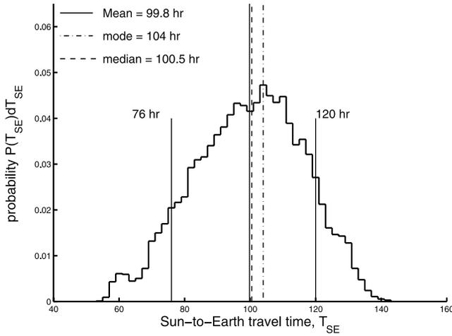
**Figure 4.** The distribution of solar wind transit times from  $r = 2.5R_s$  to  $r = R_1 = 1$  AU,  $T_{SE}$ . The full length solid vertical line gives the mean (99.8 hours), and the half-length vertical solid lines give the lower and upper decile values (76 and 120 hours). The dot-dashed and dashed lines give the mode (104 hours) and median (100.5 hours), respectively.
