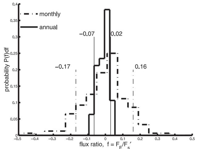
**Figure 8.** The distribution of monthly values (dot-dashed line) and annual values (solid line) of the ratio of fluxes  $f = F_E/F'_s$ . The vertical dot-dashed lines give the lower and upper decile values for monthly data ( $-0.17$  and  $0.16$ ), and the vertical solid lines give the corresponding values for the annual data ( $-0.07$  and  $0.02$ ).
