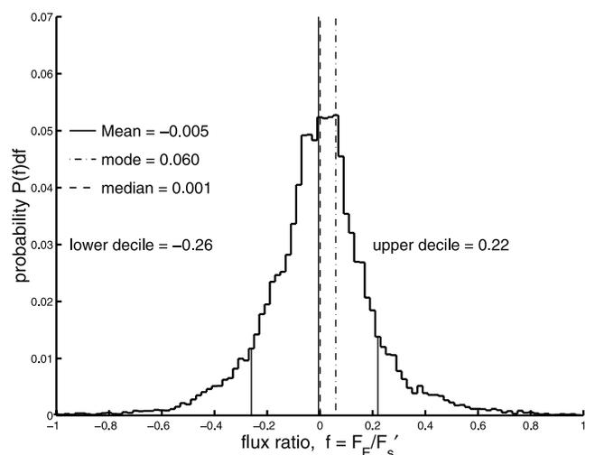
**Figure 6.** The distribution of hourly values of the ratio of fluxes  $f = F_E/F'_s$ . The full length solid vertical line gives the mean ( $-0.005$ ), and the half-length vertical solid lines give the lower and upper decile values ( $-0.26$  and  $0.22$ ). The dot-dashed and dashed lines give the mode ( $0.060$ ) and median ( $0.001$ ), respectively.
