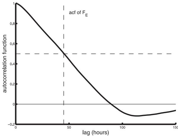
**Figure 7.** Autocorrelation function (acf, autocorrelation coefficient as a function of lag) of hourly values of the flux threading the ecliptic plane inside Earth's orbit,  $F_E$ . The dashed lines mark the lag where the acf falls to 0.5 (45 hours).
