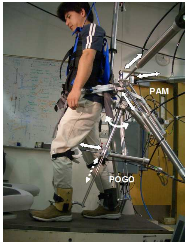
Fig. 3. PAM/POGO, two pneumatic robots used to assist gait retraining
