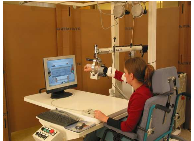
Fig. 2. Gentle/s commercial prototype for machine mediate neuro-rehabilitation
