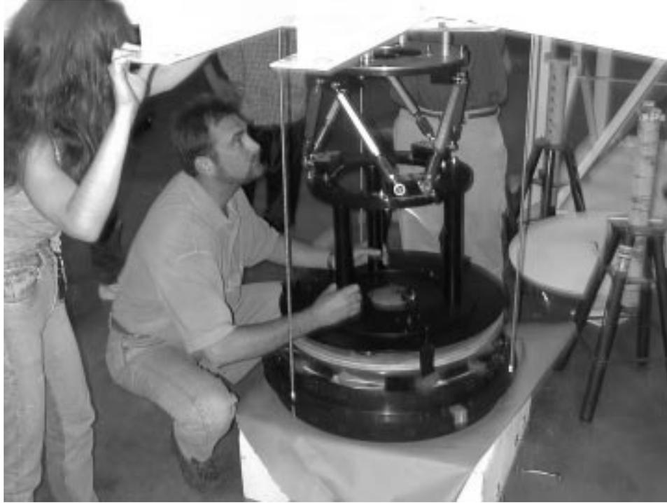
**Figure 8.** Installation of the solid dummy secondary above the two large lenses into the top part of the Shimmulator tower. The top part of the tower was then hoisted by crane to be secured atop the bottom section of the tower.
